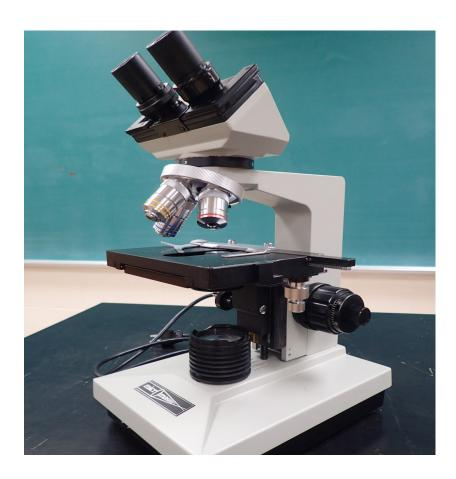
Figure XI:6 A basic compound microscope with 40x, 100x and 400x magnifications. HEM
