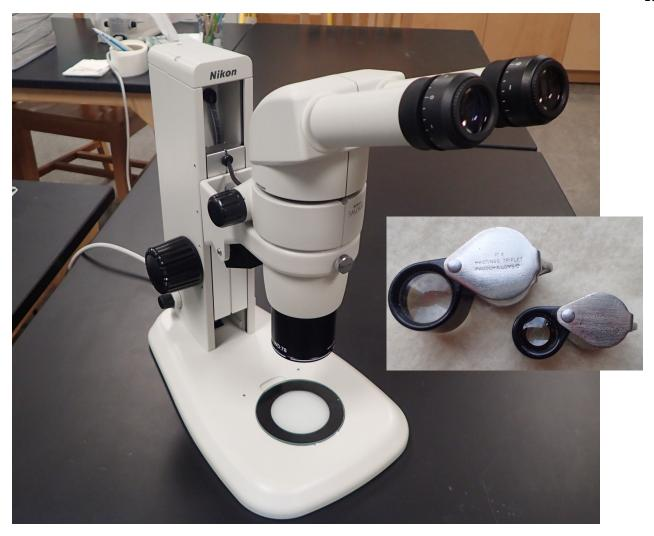
Figure XI:2 A basic stereomicroscope. Inset: A standard 10x and a 20x hand lens (loupe), essential for field examination of charophyte material. HEM
